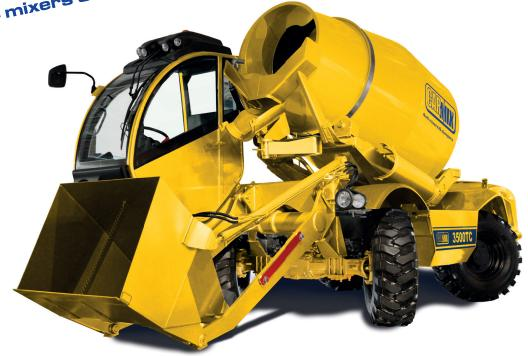
PROMIX: In-drum probe, easy allows to anayze your concrete: slump, volume, temperature and ready-mix indicator: Your on site Lab!
