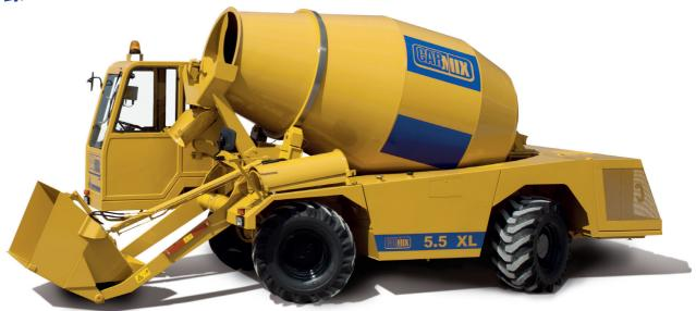
PROMIX: In-drum probe, easy allows to anayze your concrete: slump, volume, temperature and ready-mix indicator: Your on site Lab!
