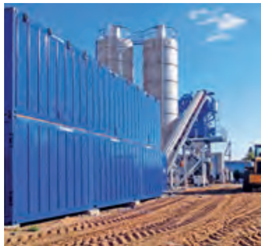
^ Semi-Mobile Batching Plant Type MCM
