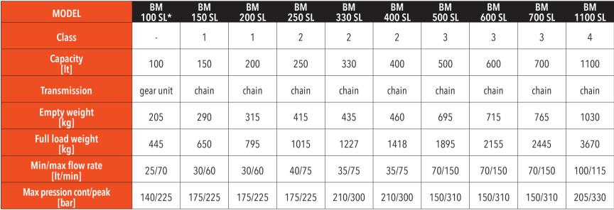
\* this mixer bucket is only available with the side discharge, without unloading pipe and electric valve.
