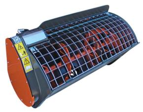
Welded helix made of wear steel HB400 Unloading pipe 1500mm lenght Sintered steel seal group
