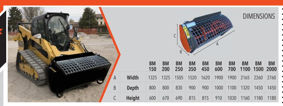
The concrete mixer bucket M3 is equipped with: BOTTOM AND HELIX made of wear resistant STEEL HB400 - Rounded fixed safety grid complete with bagbreaker - Electric valve - Hydraulic hoses - Electric connection kit - Flat Face Couplings (only on SSL) - hydraulic opening of the bottom through a cylinder with covered rod - chain tensioner - unloading pipe length mm 1500 - attachment to the machine.
